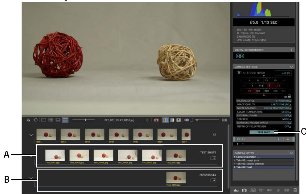
A. Test Shot Image tray. B. References tray. C. Test Shot button.
