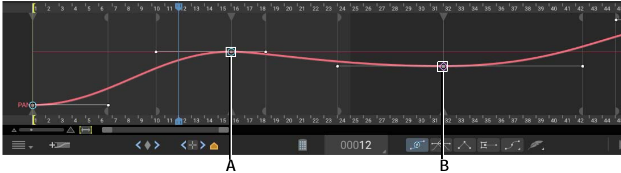
A. Blue circle around keyframe: Auto-smoothing applied. B. Purple diamond around keyframe: Auto-ease applied.
